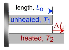
coeff. thermal expansion  $\frac{\Delta L}{L_0} = \alpha \left( T_2 - T_1 \right)$
