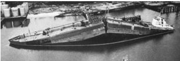
Ship-cyclic loading from waves.
