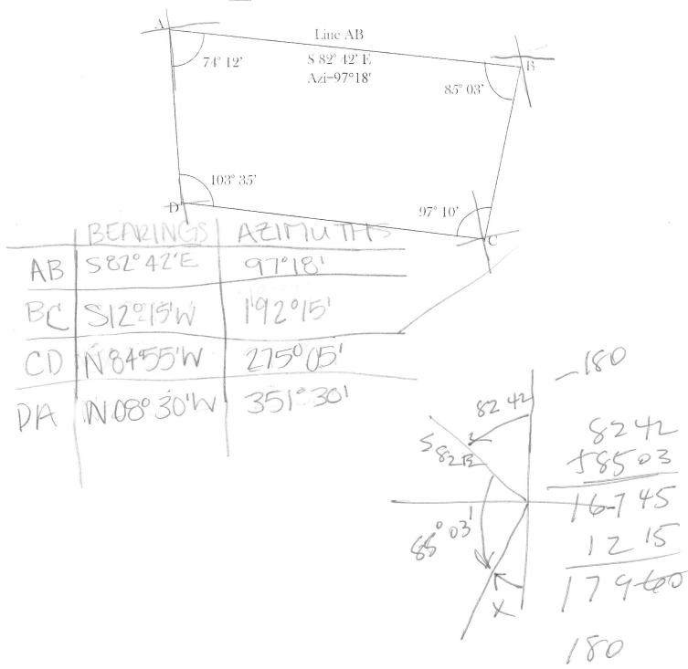
10. For the figure shown below, compute the interior angles at points A, B, and C. Show your work. Perform the appropriate mathematical check for your solution.
