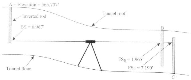
In the above figure, an elevation "shot" in an underground tunnel is shown. The backsight is taken off the tunnel roof (at point A), foresight B is taken off the tunnel roof (FS<sub>B</sub>), and foresight C is taken off the tunnel floor (FS<sub>C</sub>). Use the figure as a guide to answer the following questions. Hint: The positive backsight computation method typically used in differential leveling will not work in this problem. Important: Show your work.
