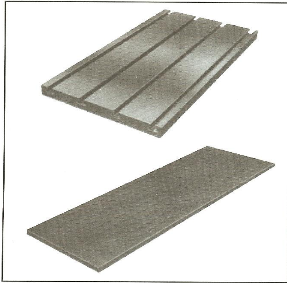
Figure 11-9. Subplates. (Courtesy Mid-State Machine Products)
